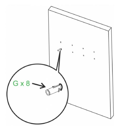
3. Install the (A) wall mount frame onto the wall by securing the eight (F) wall screws and (E) washers to the anchors.
