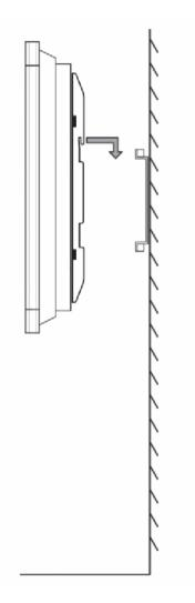
5. Secure the wall mount brackets to the frame using the two (D) frame screws.
