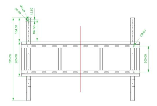
Wall Mount Frame dimension / units of length are "mm"
