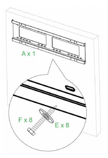
4. Mount the displays' wall mount brackets onto the wall mount frame.
