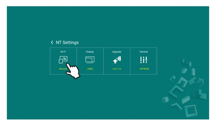
There are four connection types on NC-X500: Miracast mode, Wi-Fi Hotspot, connect to Wi-Fi, and turn off Wi-Fi to use Ethernet only.
