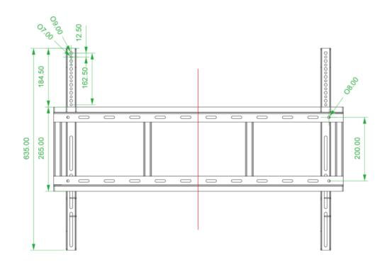
Wall Mount Frame dimension / units of length are "mm" A: Wall Mount Frame x1 B: Wall Mount Brackets x2 C: Bracket Screws x6 ( M8 x25mm , 4 pcs are recommended for installation ) D: Frame Screws x2 (M5x60mm) E: Wall Screw Washers x8 ( Φ16 x 8.3×1 mm , 6 pcs are recommended for installation ) F: Wall Screws x6 (Φ8 x 55 mm , 8H , 6 pcs are recommended for installation) G: Anchor Screws x6 (Φ10x 49.5 mm , PP, 6 pcs are recommended for installation)
