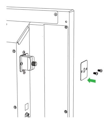
3. Attach the external antenna securely to the screw-on stud.
