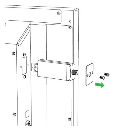
2. Secure the cover with screws. Make sure the antenna screwon stud is positioned and exposed properly.
