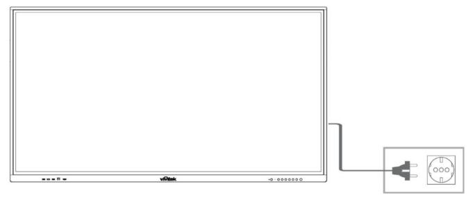
Step 2. Turn the power switch located at the right side of the display on.
