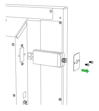
2. Secure the cover with screws. Make sure the antenna screwon stud is positioned and exposed preperly.
