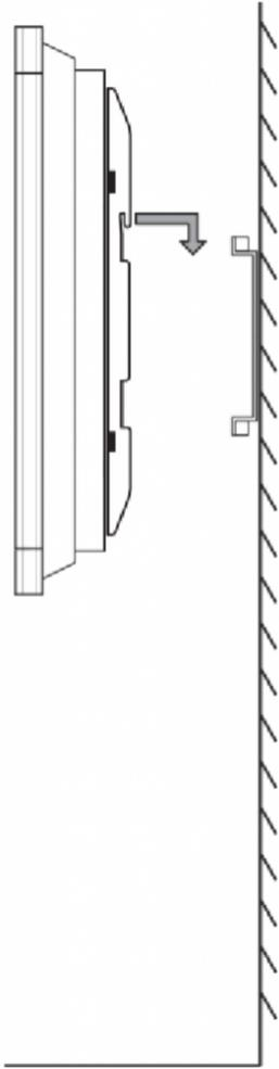
5. Secure the wall mount brackets to the frame using the two (D) frame screws.
