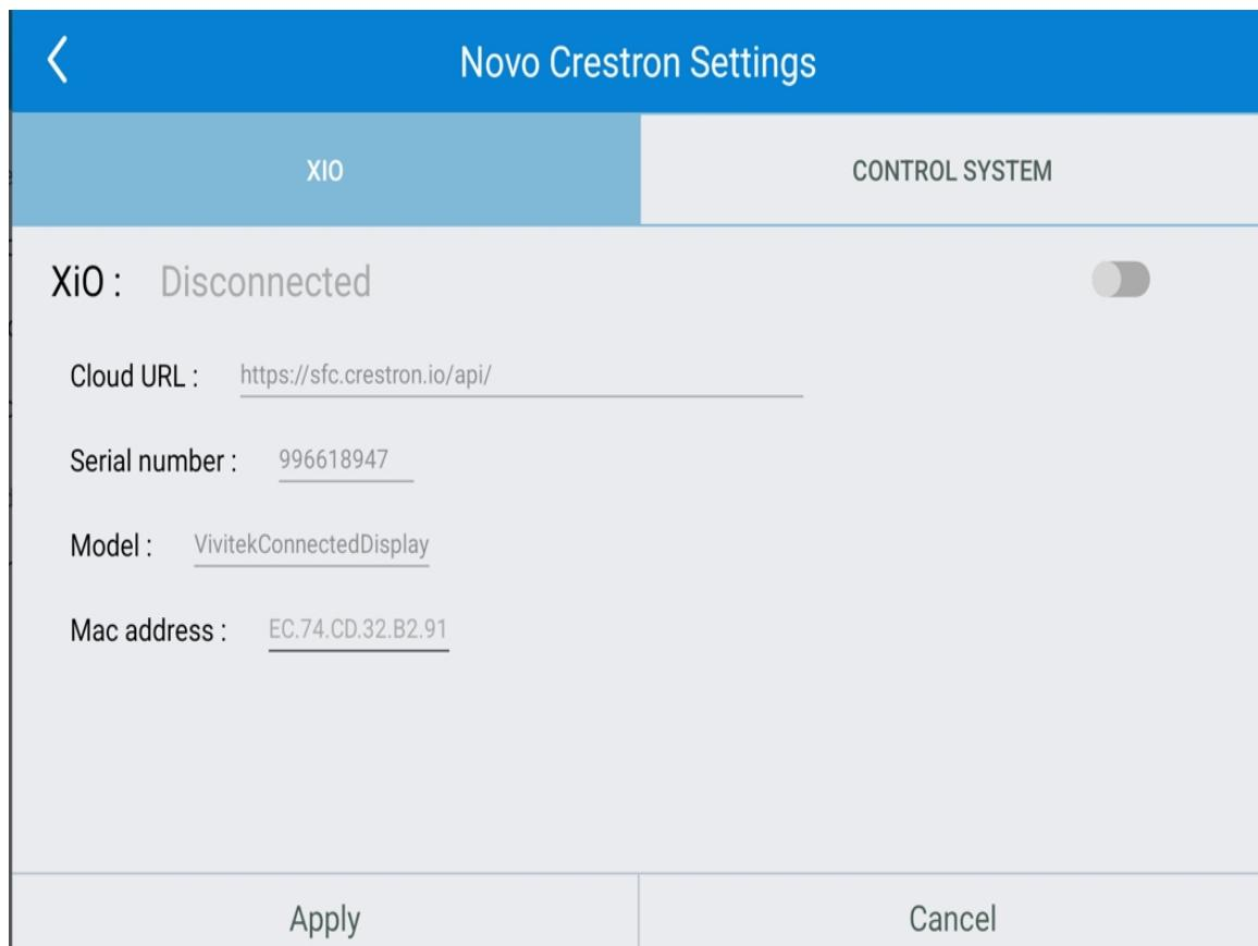
Step 7. The second tab is **Control System**. Fill in the required information or enable **Auto Discover**, then click **Apply** to connect to a **local Crestron system**.
