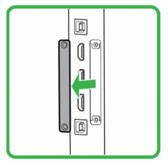
3. Insert the Wi-Fi module into the slot.
