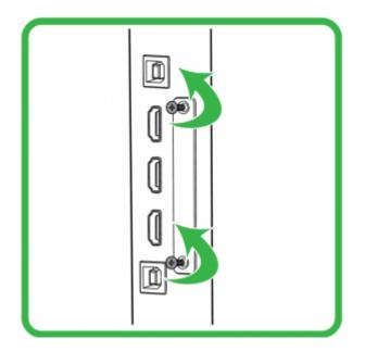
2. Remove the Wi-Fi module slot cover.
