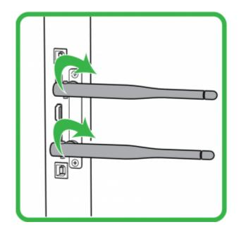
Installing the Wi-Fi module (EK-3 series)
