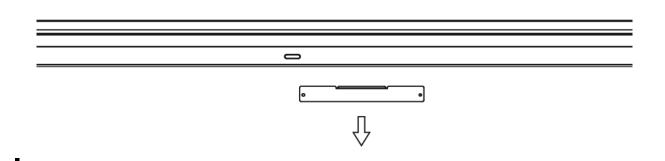
2. Insert the WiFi module fully into the NovoTouch along the direction of the arrow.
