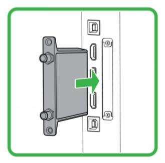
4. Install the two screws to secure the Wi-Fi module to the display, and then install the antennas onto the Wi-Fi module.
