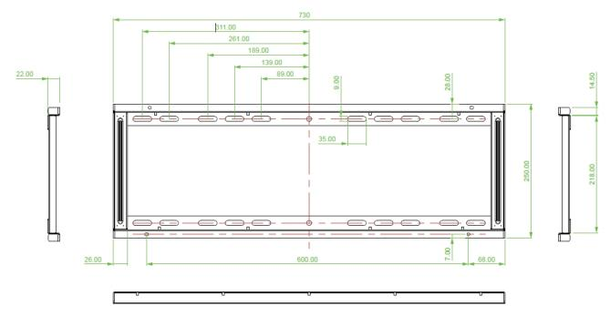
$65\ensuremath{^{\prime\prime}}$  wall mount bracket dimension / units of length are "mm"
