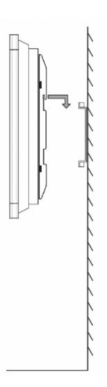
5. Secure the wall mount brackets to the frame using the two (D) frame screws.
