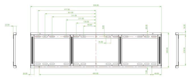
75" & 86" Wall Mount Frame dimension / units of length are "mm"
