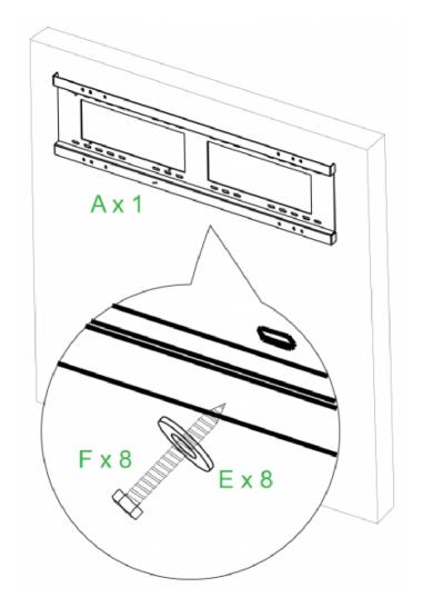
4. Mount the displays' wall mount brackets onto the wall mount frame.
