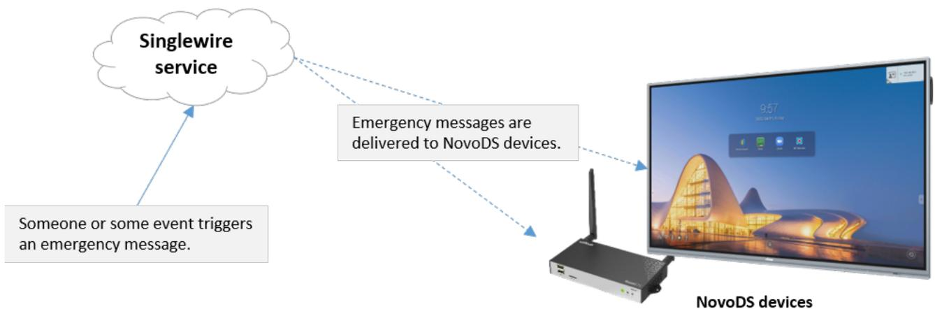
The remaining section describes the basic concept and setup instructions of setting up Singlewire on NovoDS devices.
