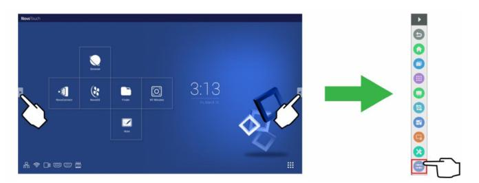
Once the input source menu is open select the video input you want to show on the display. Video inputs with a blue dot underneath indicate video inputs that are currently connected.
