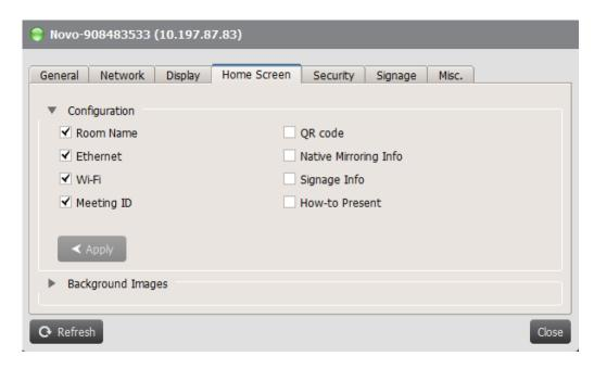
**Modify Home Screen Picture**: NovoConnect X500 and NovoDisplay can customize background picture, user can upload picture to change home screen background.
