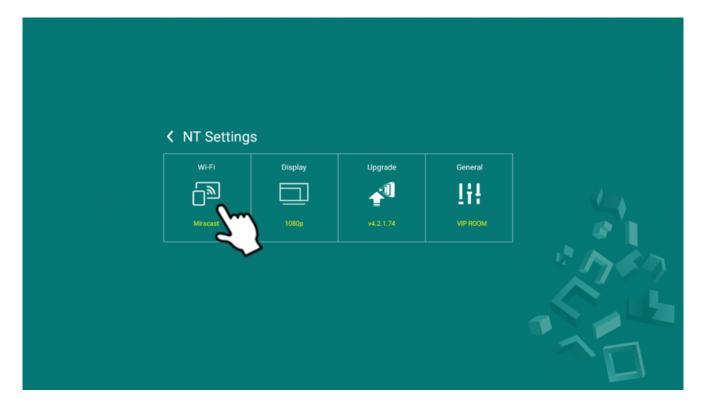
There are four connection types on NC-X900 and NC-X700: Miracast mode, Wi-Fi Hotspot, connect to Wi-Fi, and turn off Wi-Fi to use Ethernet only.
