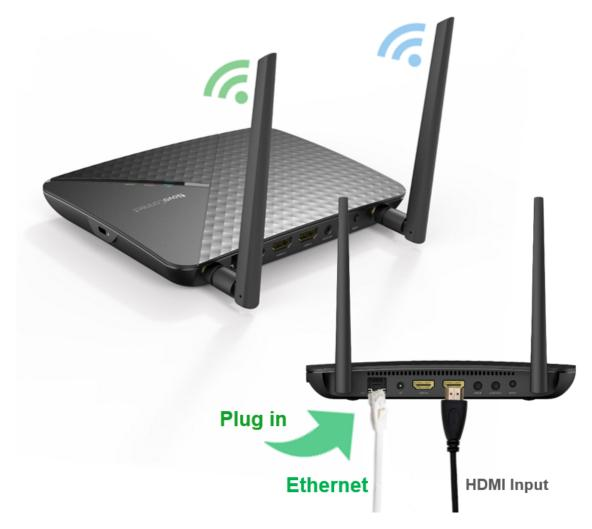
NovoConnect NC-X700 and NC- X900 can be plugged into Ethernet via its RJ45 port. User can connect to organization's backbone network. It is recommended to use Ethernet connection (when possible) since it gives you better robustness and higher performance.
